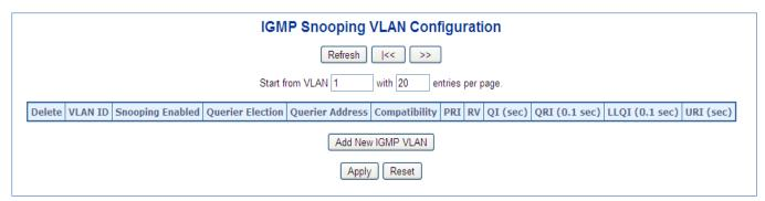
Figure 4-3-9-8: IGMP Snooping VLAN Configuration Page Screenshot
