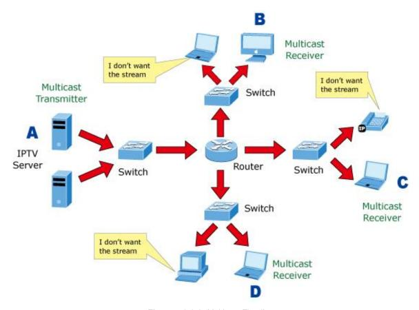
Figure 4-3-9-2: Multicast Flooding
