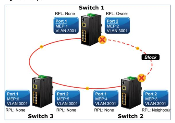
Figure 4-6-4-2: Ring Example Diagram
