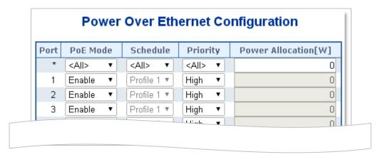
Figure 4-8-4-1: Power over Ethernet Configuration Screenshot
