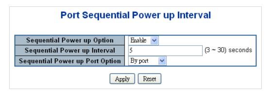
Figure 4-8-6-1: PoE Port Sequential Power Up Interval Configuration Screenshot
