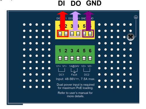
Figure 2-1-22: Wiring the DI and DO of IGS-6325 Din-rail Series.
