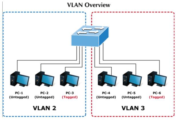
Figure 4-3-3-7: Two Separate VLANs Diagram
