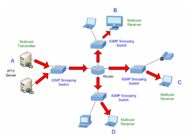
Figure 4-3-9-3: IGMP Snooping Multicast Stream Control
