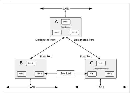
Figure 4-3-8-3: After Applying the STA Rules
