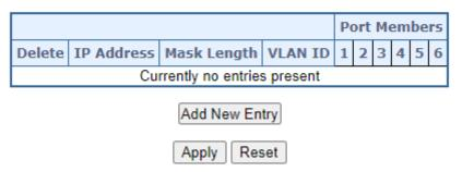
Figure 4-3-5-2: IP Subnet-based VLAN Membership Configuration
