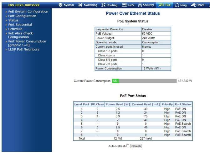
Figure 4-8-1-1: Power over Ethernet Status
